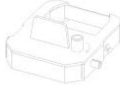
Installing the ribbon cartridge so that the ribbon is between the print head and ribbon mask.
