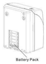
(4) Insert the lid into the slot, keep pressing it down until it hooks to the clasp.
