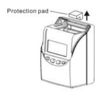
(3) Unlock with key and remove the top cover.
